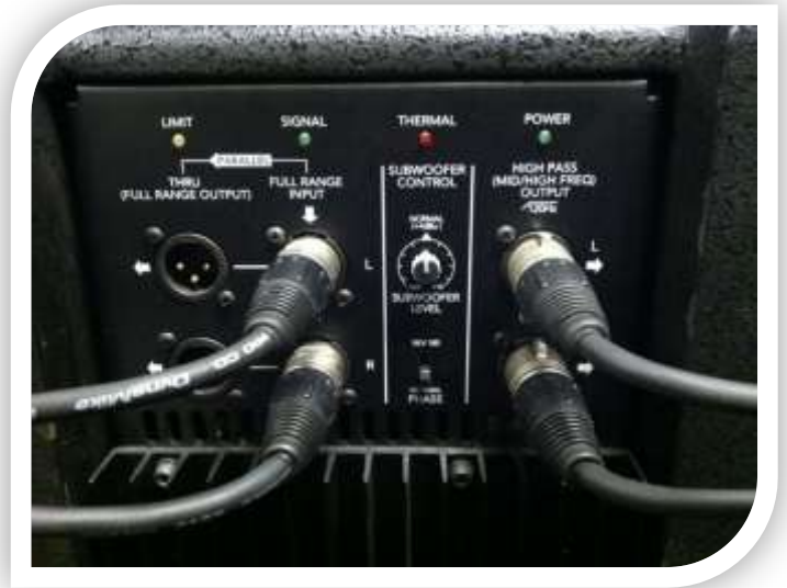
Sub Wiring " MIXER OUTPUT to FULL RANGE INPUT , HIGH PASS OUTPUT connects to speaker INPUT "
