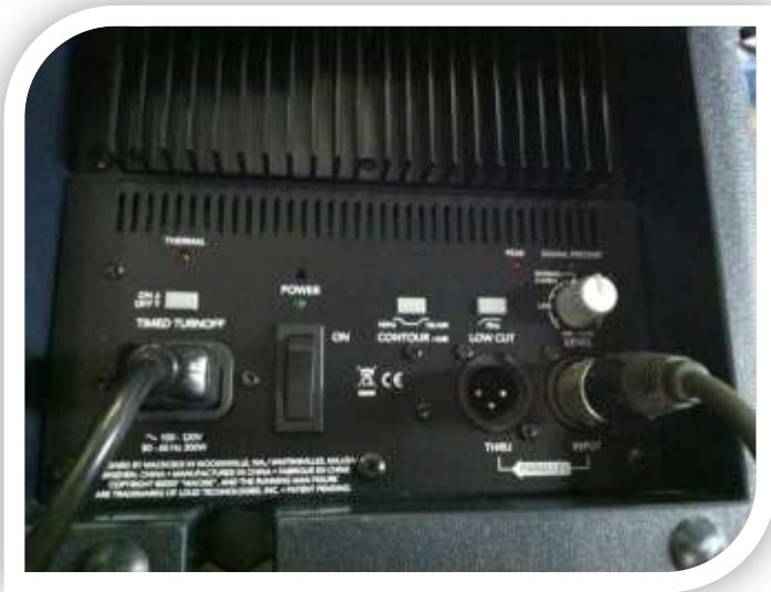
Speaker wiring " MIXER OUTPUT connects to INPUT "
